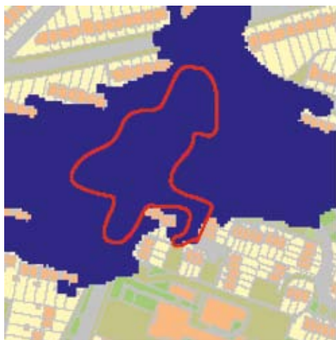
a) 2D overland routing of uniform rainfall event
